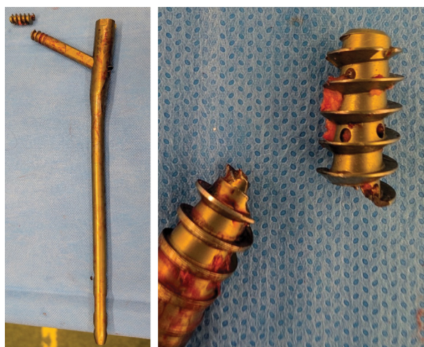
Figure 5: Explanted implant showing break through the thread fenestrations.
